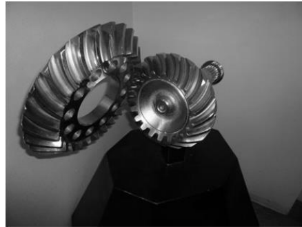
Fig. 3. Crown wheel (left) and pinion (right).
