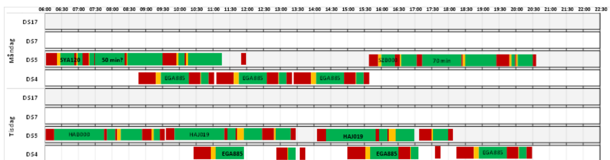
Fig. 4. New schedule for two days in two machines manned by one operator.
