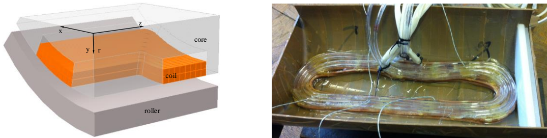
Fig. 8. Section of an excitation coil placed against the cylindrical work piece (left), and practical realization of inductor for in-roll heater (right).
