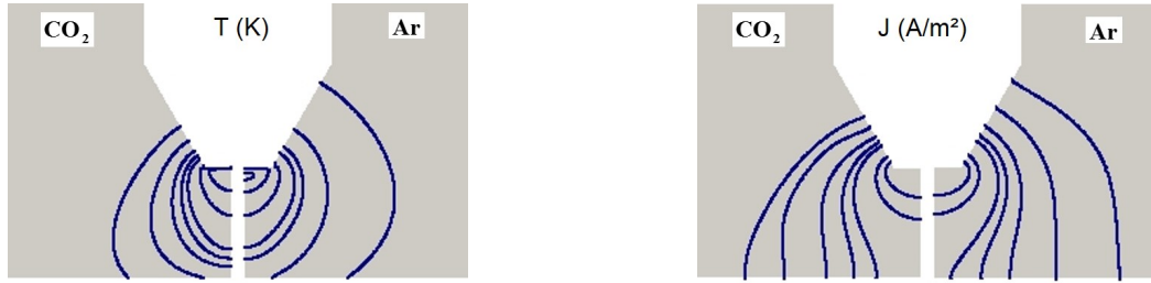
Fig. 4. Zoom of contours between electrode and base metal. Left: temperature T and Right: current density J (with \text{CO}_2 in each left section, \text{Ar} in right section). From large to small radius the T -contours (resp. J -contours) correspond to 12, 14, 16, 18, 20, 22 and 24 kK (resp. 1, 2.5, 5, 7.5, 10, 25, and 50 MA/m 2 ).
