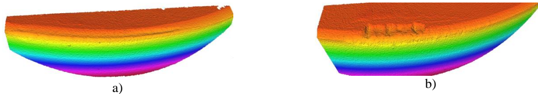
Fig.8. Comparison of tool wear for different tools when machining hardened high C-Si HCCl at v_c = 160 m/min: a) BCBN; b) HCBN.
