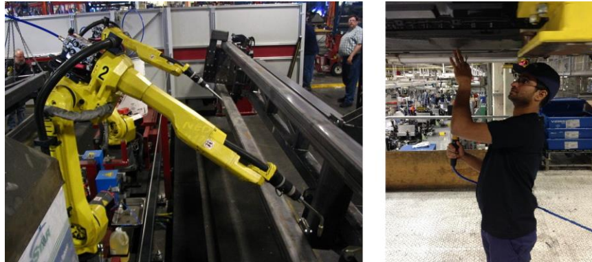
Fig. 1. An ABB industrial robot welds Body in White parts (Volvo Cars 2014) which is a completely automated process in most car assembly plants (left). A line worker performing final assembly using a power assist device (right).
