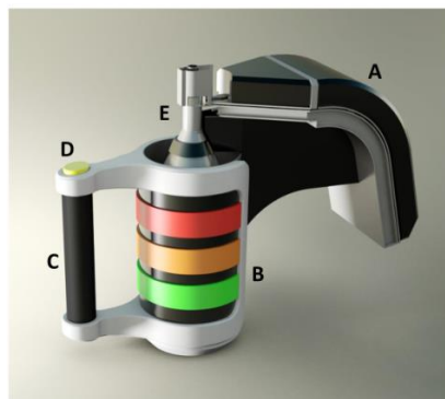
Fig. 4. Rendering of an automated bolt fastener (Left). The end effector mounted on a test robot – Yaskawa Motoman SIA20D (Right).
