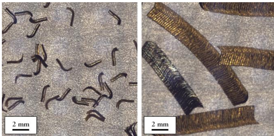
Fig. 7. Comparison of obtained chips while machining CuZn39Pb3 (left) and CuZn21Si3P (right) at f = 0.20 \text{ mm/rev} and a_p = 2.0 \text{ mm} .
