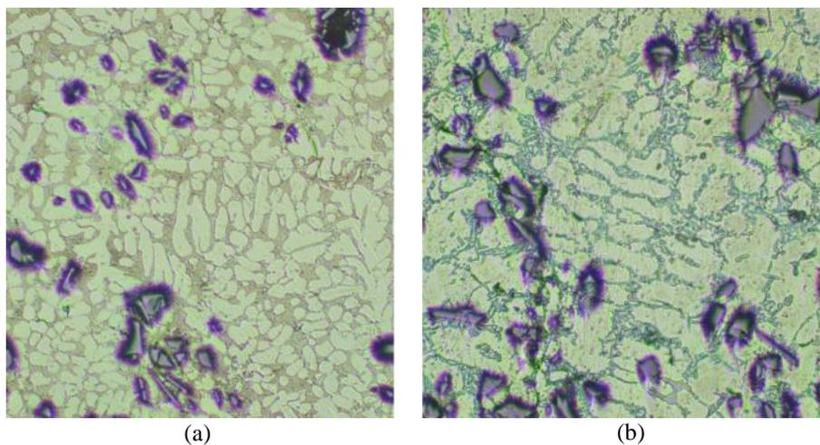
Fig. 3. Microstructure of the sample cast at room temperature (a) and 350°C (b), both at 200X magnification.
