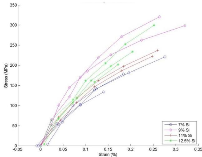
Fig. 8. Tensile strength depending on matrix silicon content.
