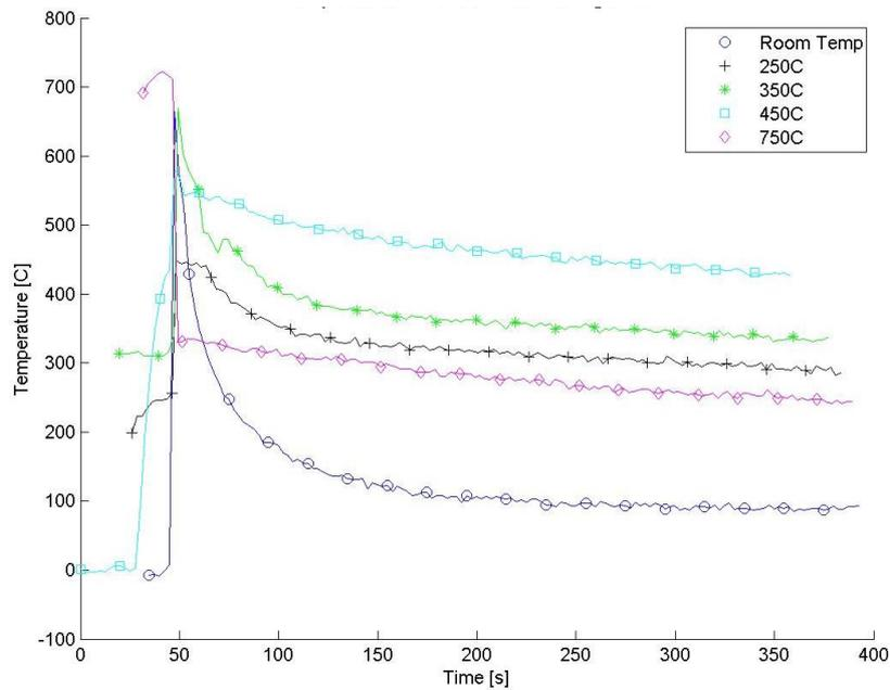
Fig. 2. A comparison between the temperature curves for the different cast samples.
