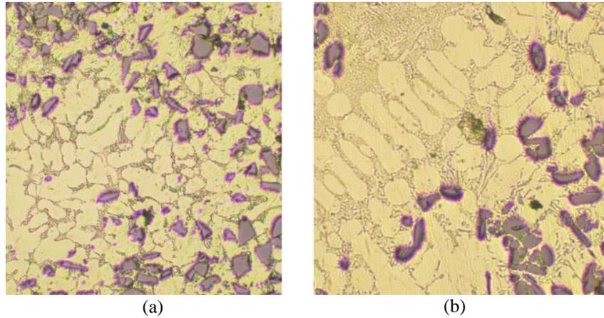
Fig. 6. Microstructure 7 % Si (a) and 11 % Si (b), both at 200x magnification.
