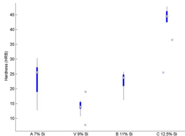
Fig. 7. Hardness for varying silicon content.
