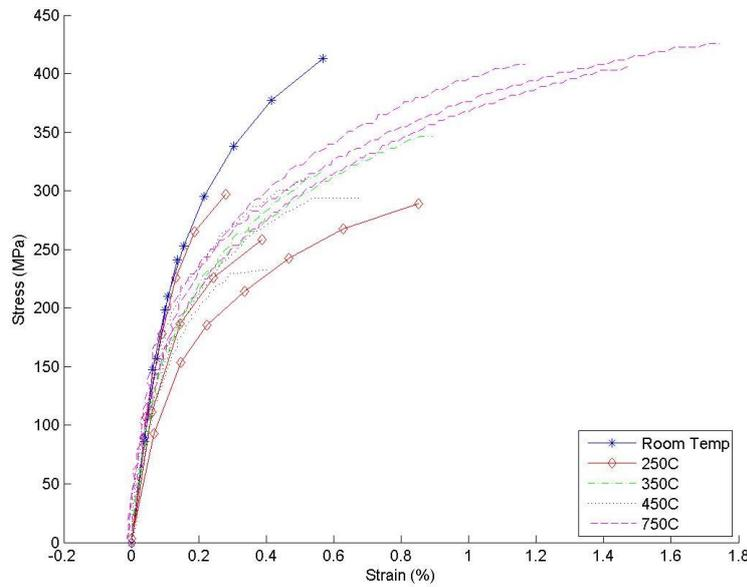
Fig. 4. Tensile strength dependent on cooling rate.
