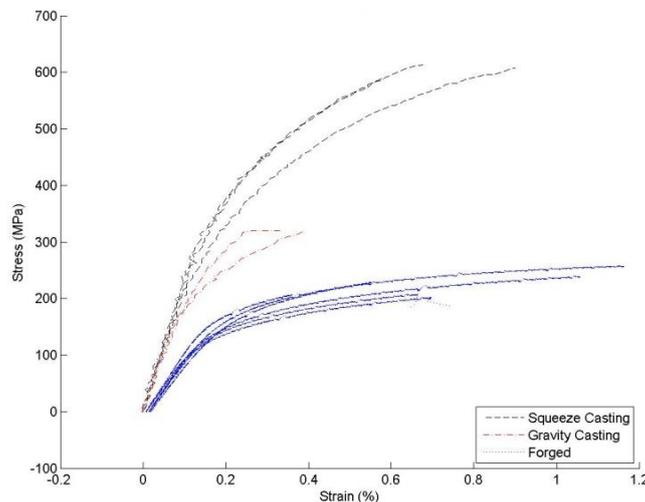
Fig. 9. A comparison material strength manufactured by different methods.
