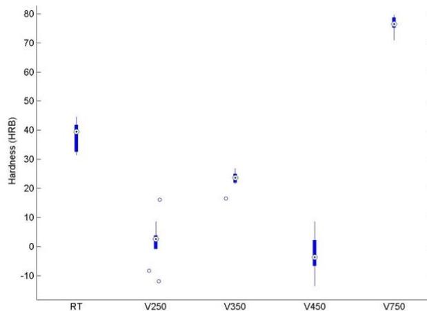
Fig. 5. Hardness for varying mold temperature.
