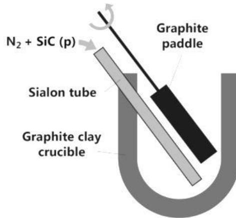
Fig. 1. A schematic view of the SiC introduction technique.
