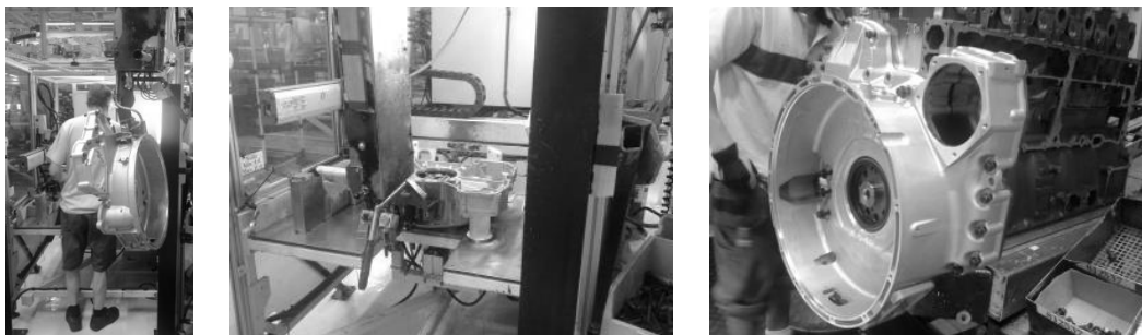
Fig. 2. Assembly sequence: Lift flywheel cover, put cover in an automated silicon applying machine and aid the assembly operator when assembling cover on engine block by carrying the heavy load.
