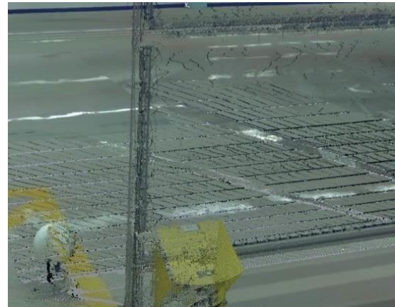
Fig. 11. Quality problems with scanning a lattice.
