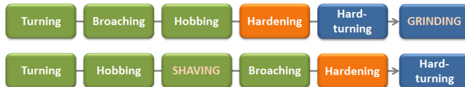
Fig. 1. The major manufacturing steps in a gear wheel manufacturing, were the value stream at the top contains grinding and the value stream at the bottom contains shaving.
