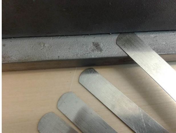
Fig. 3. Thickness gauges used to measure gap size.
