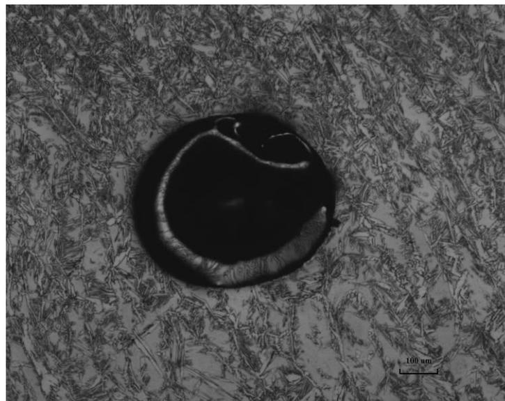
Fig. 6. Micrograph of sample SD 7 showing a pore of around 0.5 mm diameter.
