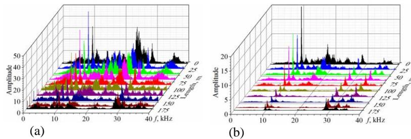
Fig. 4. Spectra of acceleration signals change in the cutting length for pcBN (a) and bcBN (b) tool grades.
