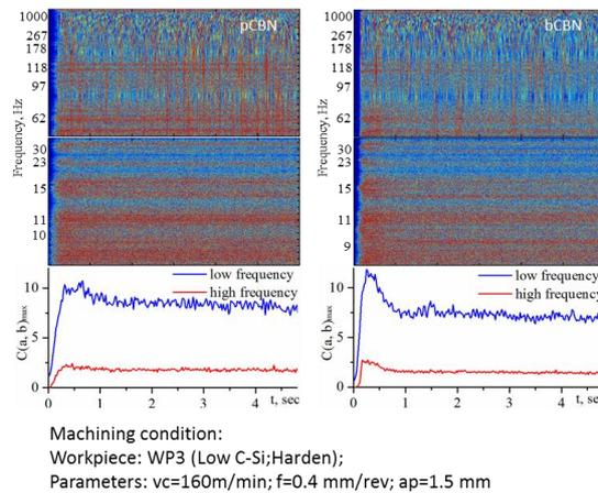
Fig. 5. Wavelet analysis of vibration signals measured when machining with pcBN and bcBN tools.
