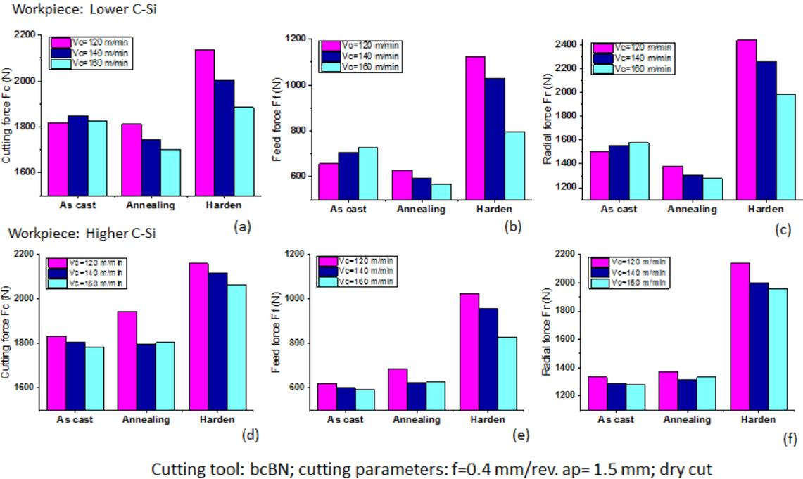
Fig. 3. Cutting forces produced by bcBN tools when cut two groups of materials under three cutting speeds.
