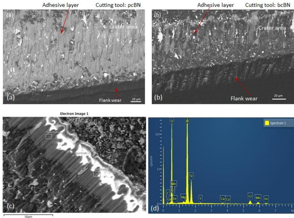
Fig. 8. Adhesion layer generated on pcBN tool (a) and bcBN tool (b) during machining high Cr white casting iron; EDX analysis of adhesion layer on tool wear region (a) and (d).
