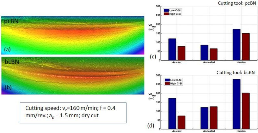
Fig. 7. Flank wear and crater wear on pcBN and bcBN cutting tools in (a) and (b); wear rate generated on pcBN and bcBN tools when machining six different materials in (c) and (d).
