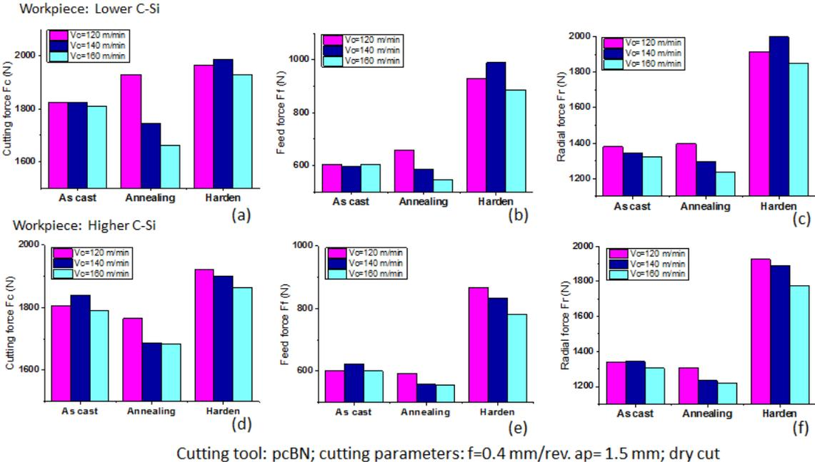
Fig. 2. Cutting forces produced by pcBN tools when cut two groups of materials under three cutting speeds.
