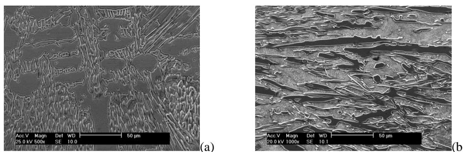
Fig. 1. Microstructure of high Cr white cast iron (as-cast): (a) lower C-Si contents and (b) higher C-Si contents.
