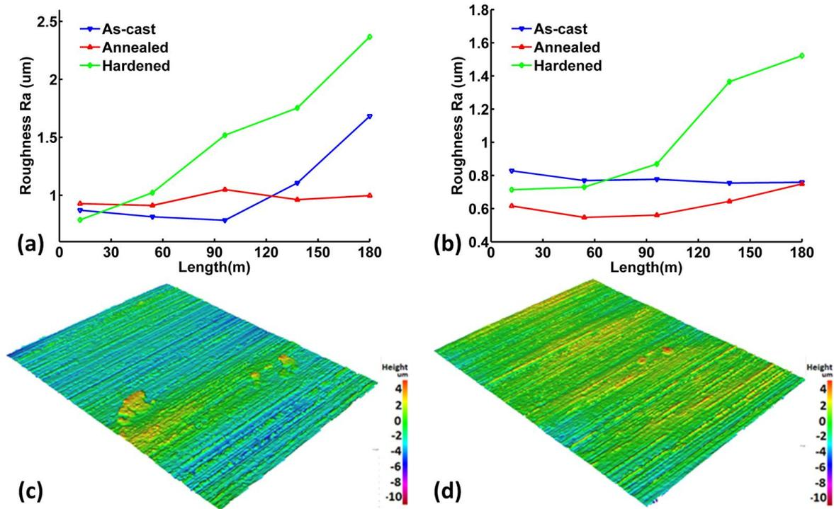
Fig. 6. Surface roughness  $R_a$  and 3D surface profile produced by pcBN and bcBN cutting tools on as-cast materials in higher C-Si.
