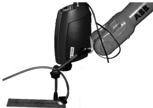
Fig. 1. Image of demonstrator for inspection of surface cracks. The emissivity varitiation detected by the IR camera is fed to the robot for positioning during inspection.
