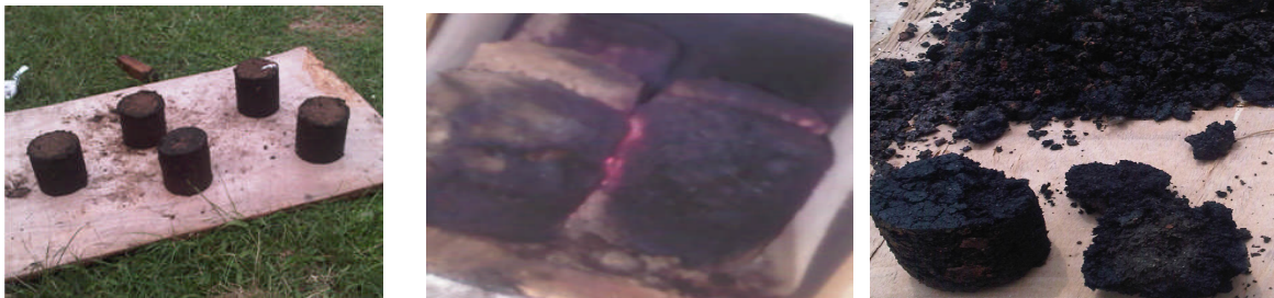
Fig 1: Extruded briquettes being air dried (Left picture) and activated in a furnace (central picture) for production of activate carbon (right picture).
