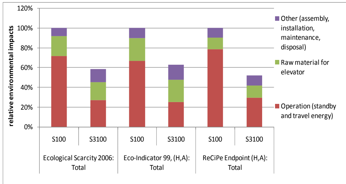
Figure 3: Comparison of the environmental impacts from the old lift (S100) and its successor (S3100)
