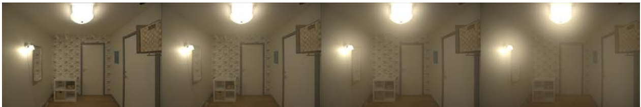
Figure 8. Light setting 1 with simulation of increased light scattering; 0%, 20%, 40% and 60%, respectively.
