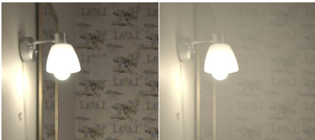
Figure 11. Light setting 1 with simulated light scattering; 0% in left picture and 40 % in right picture. Contrast measurement in the HDR image on the test symbol chart, shows that the contrast drops from 11% to 3% in presence of light scattering.
