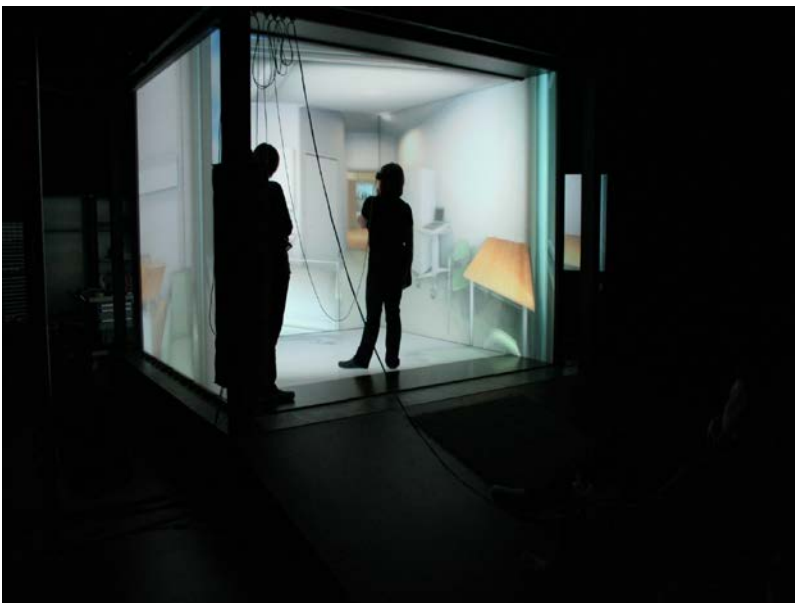
Figure1. CAVE and its surroundings (Photo by Esa Nykänen)
